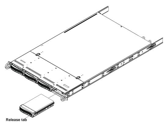
Figure 6-4. Removing a Drive from the Server
